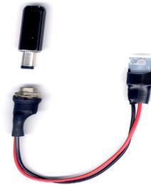
Solder an inline fuse holder in the red (positive) wire,
