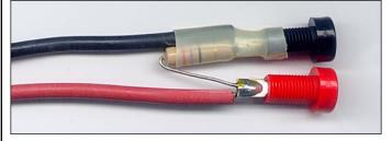
Cover the resistor and the threaded portions of the banana jacks with heat shrink tubing or electrical tape. Slip the banana plug covers up the red and black wires in preparation for connecting the plugs. Solder the banana plugs to the red and black wires and screw on the covers.
