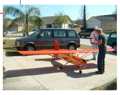
is in 2 pces as well. There are 8 HiTek HS755HB servos. One will work a brake setup he will be installing. There are flaps connected to spoilers as well.
