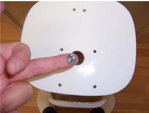
5) Thread your mounting bolt into the blind nut while still holding in position and then give it a firm tug to sink the barbs of the blind nut into the firewall.
