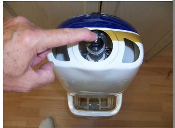
3) Center the engine (which has now been mounted on the engine brackets) in the cowl. Holding the engine in place,
