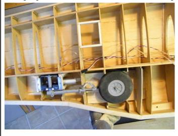
servos in the bays where the bellcranks should be and now I need to sheet the bottom of the wings and glue and shape the wing tip blocks in place to complete the wings. Oh! And the Flaps which are enormous and the Aelerons are hinged with hinge points and fitted. Same set up for the Elevators and Rudder
