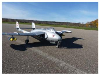
This ARF imported from Switzerland and in Swiss Airforce colours has retacts with servo operated doors and flaps and will soon have a scale cockpit. The original 6 blade EDF has been replaced with a
