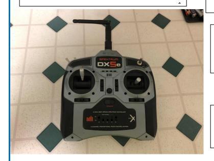
Spectrum 5 Channel Dx5e transmitter which takes 4 AA Batteries.
