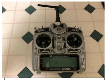
9 Channel JR 9303 Transmitter with researchable 9.9V 1500 mAh LiFe Hobby King Transmitter battery.
